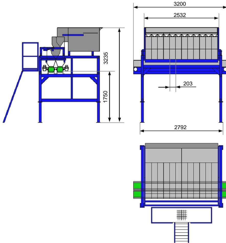
The high precision weigher Upmatic 2112DV can be combined with all current filling and sealing machines. Upmann also supplies the associated feed belts as well as processing equipment to make up complete
