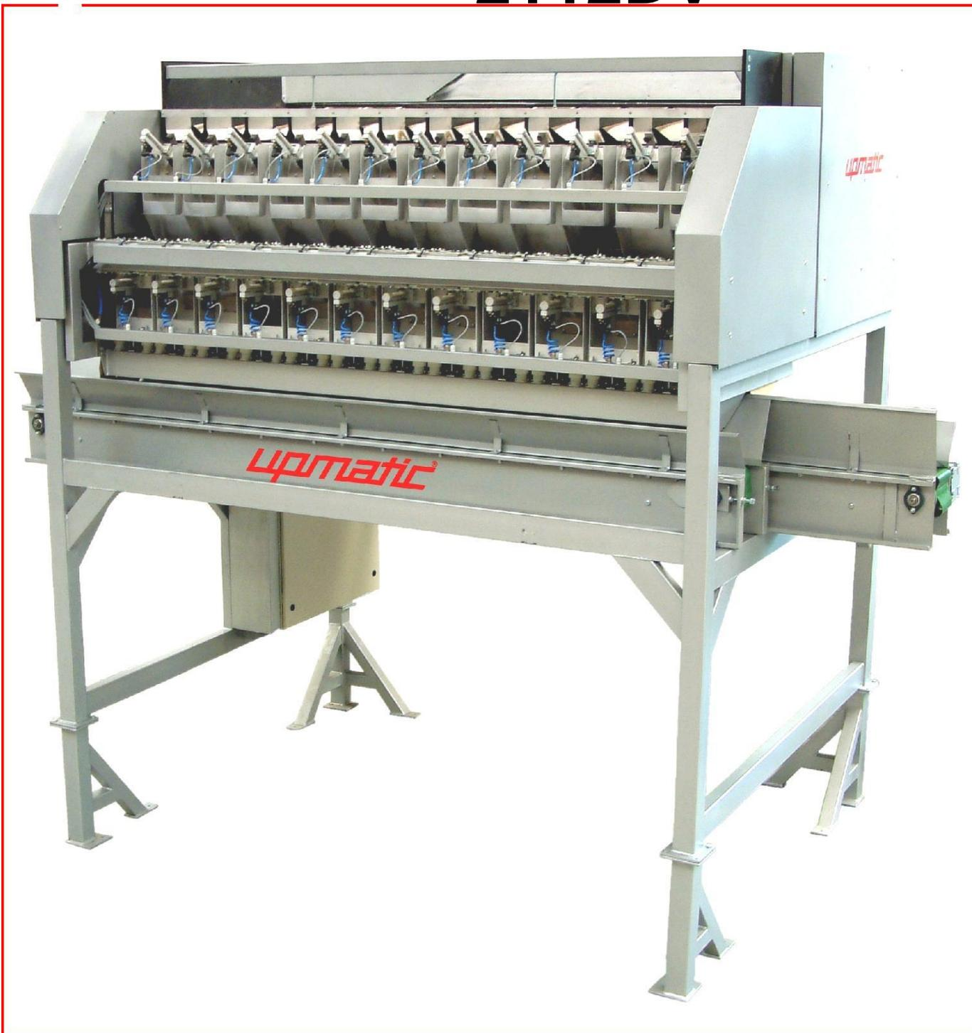
**Upmatic Type 2112DV = computer controlled proportioning component weighing machine for fine and coarse products in the food and non-food industries. The weighing range covers, dependent on product, all weight classes from 0,5 up to 25 kgs (Weighing without losses).**
