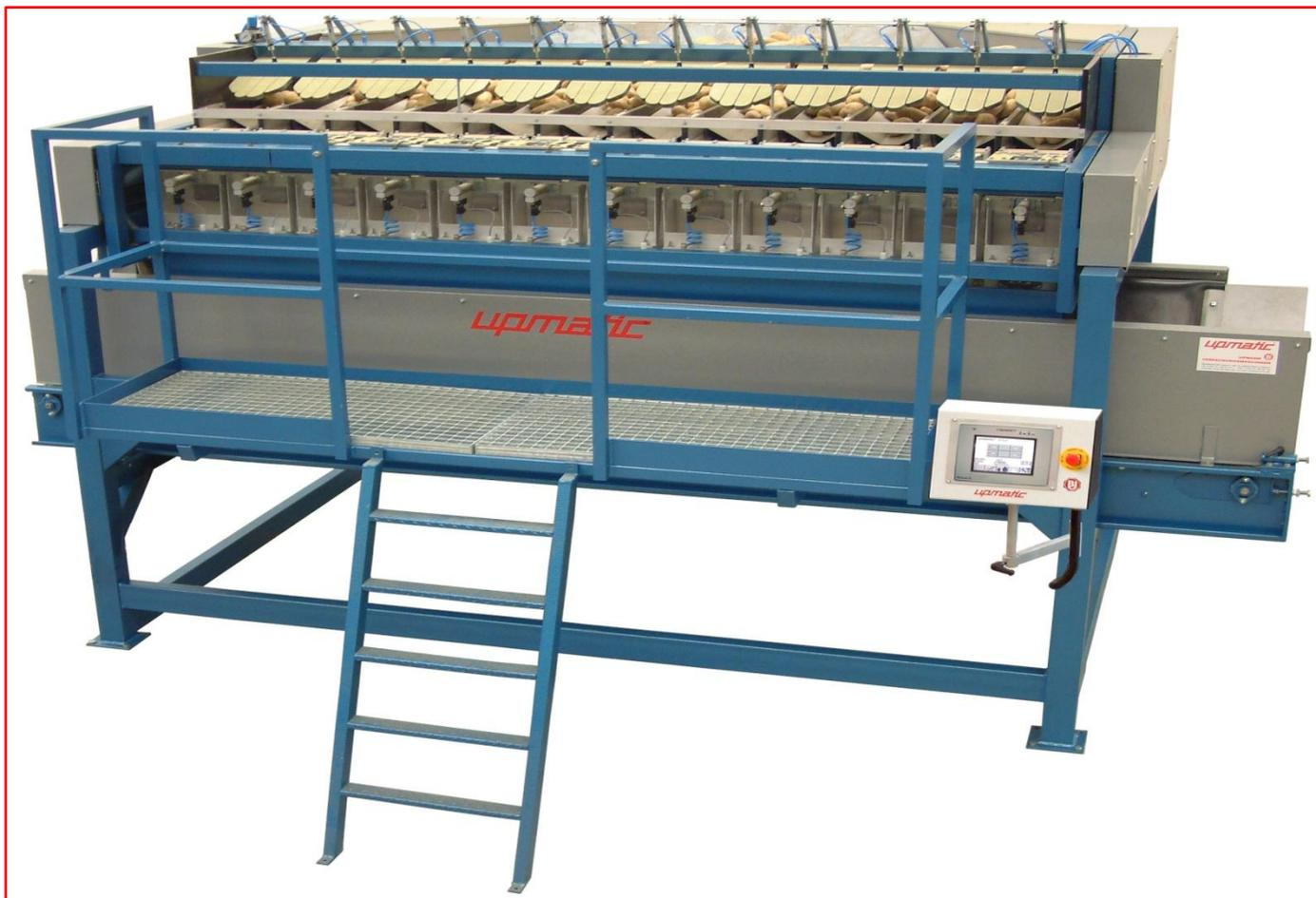
**Upmatic Type 2112 = computer controlled proportioning component weighing machine for fine and coarse products in the food and non-food industries. The weighing range covers, dependent on product, all weight classes from 0,5 up to 25 kg (Weighing without losses).**
